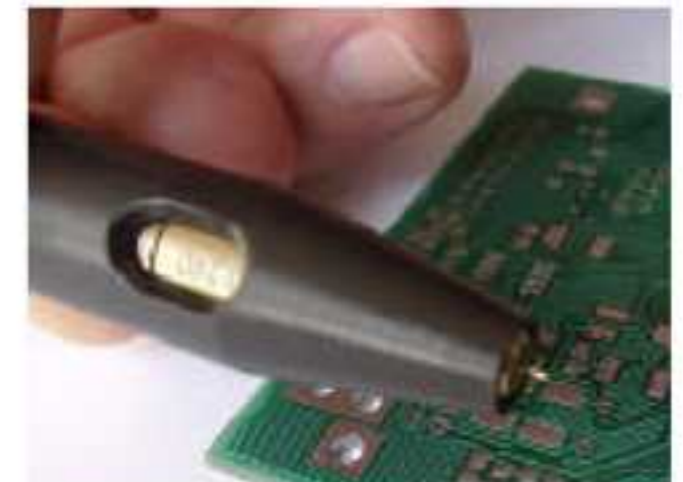
Probe EP-20, for extra smallest PTH thickness
